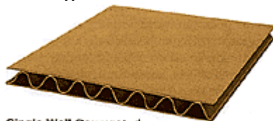
Single Wall Corrugated (also known as Double Faced)
